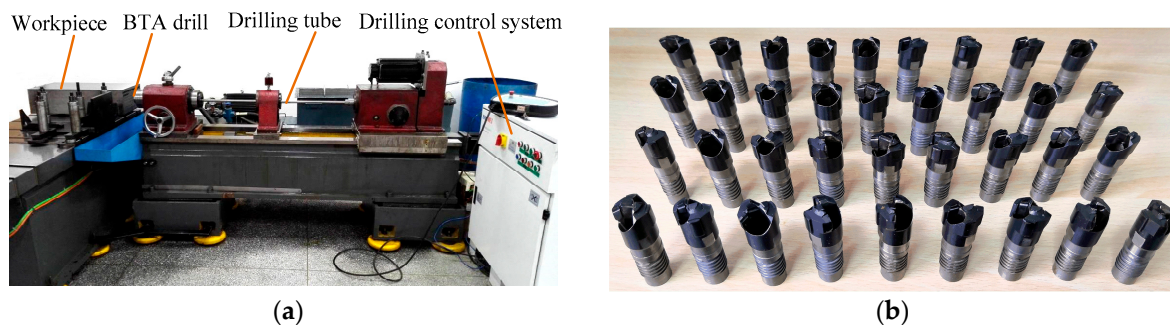
Figure 3. (a) Experimental platform and (b) staggered teeth BTA drill.
