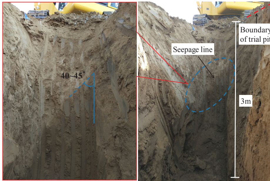
Fig. 11. The pattern of seepage line in shallow layer (imaged by authors).
