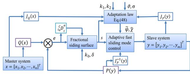
FIGURE 1. The control diagram of the generalized synchronization.
