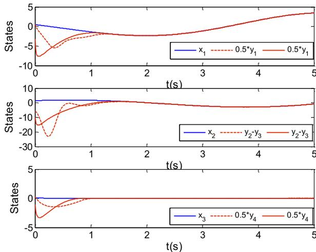
**FIGURE 5. Synchronized states of the systems (50) and (51). (Solid lines: Fixed time method; Dashed lines: Finite time method).**
