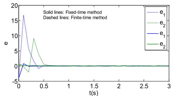
FIGURE 3. Time responses of synchronization errors (47).
