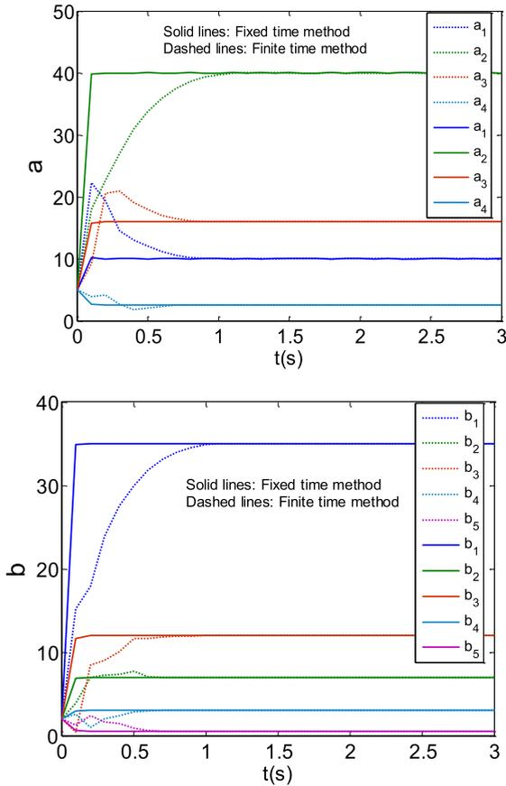
FIGURE 4. Time evolution of the adaptive parameters  $\hat{a}_i$  ( $i = 1, 2, 3, 4$ ) and  $\hat{b}_i$  ( $i = 1, 2, 3, 4, 5$ ).
