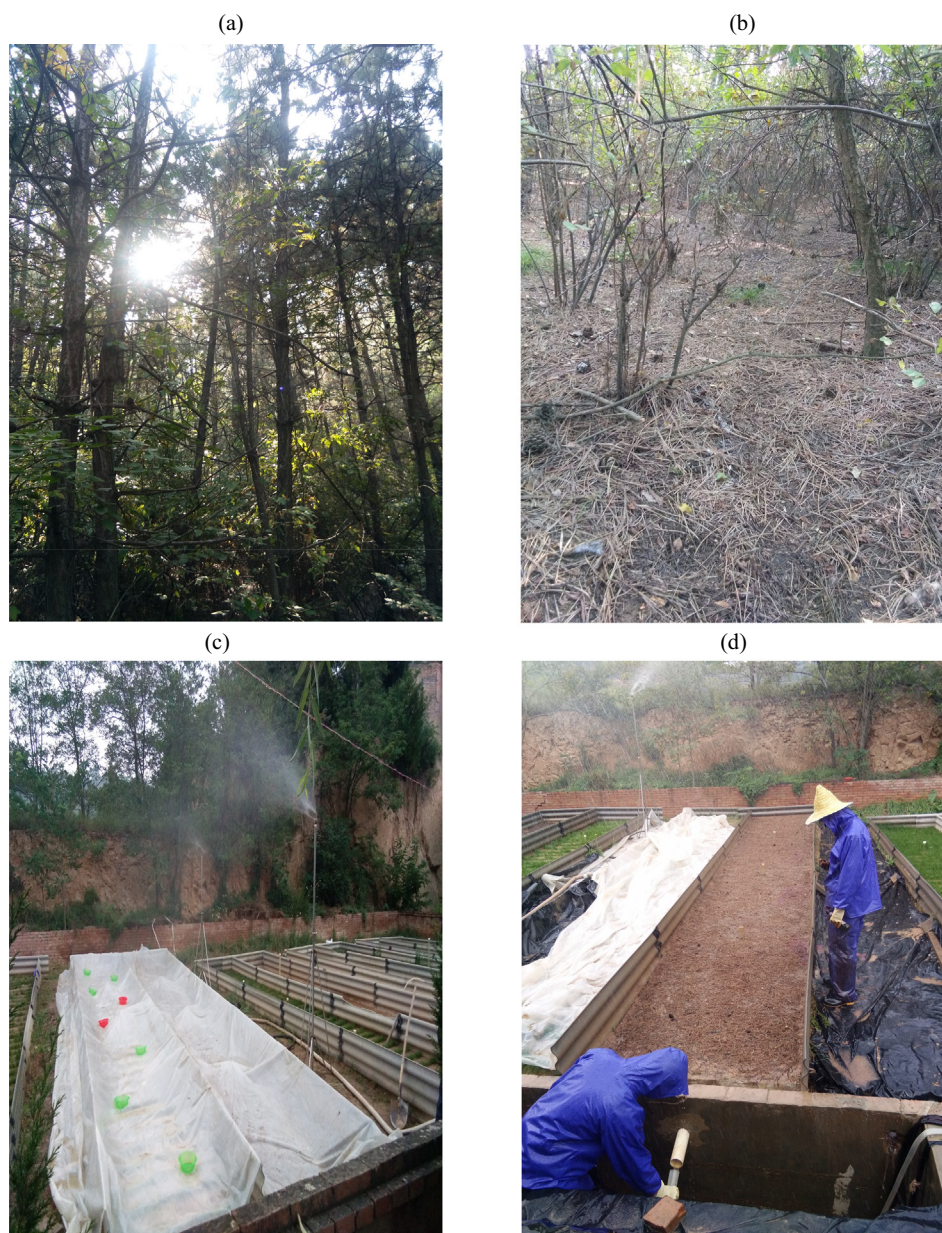
Fig. 1. Site diagram: (a) The selected P. tabulaeformis plantation stand for litter collecting; (b) litter layer covering on the P. tabulaeformis plantation stand; (c) calibration of rainfall intensity in the field plots; (d) rainfall simulation experiment conducted under a P. tabulaeformis litter mass of 500 \text{ g m}^{-2} .
